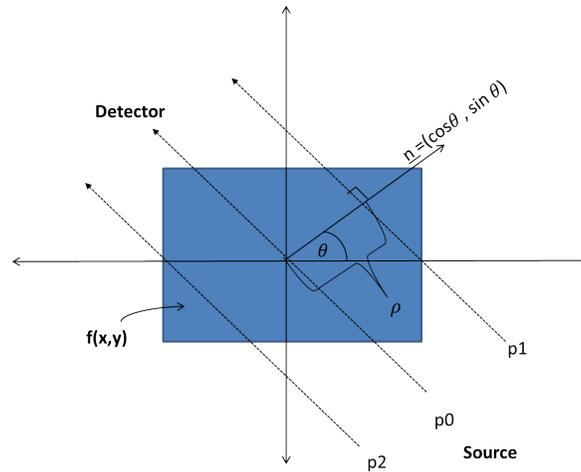
Figure 1: The figure represents parallel beams from a source to a detector through an object  $f(x,y)$  at the specific angle  $\theta$
